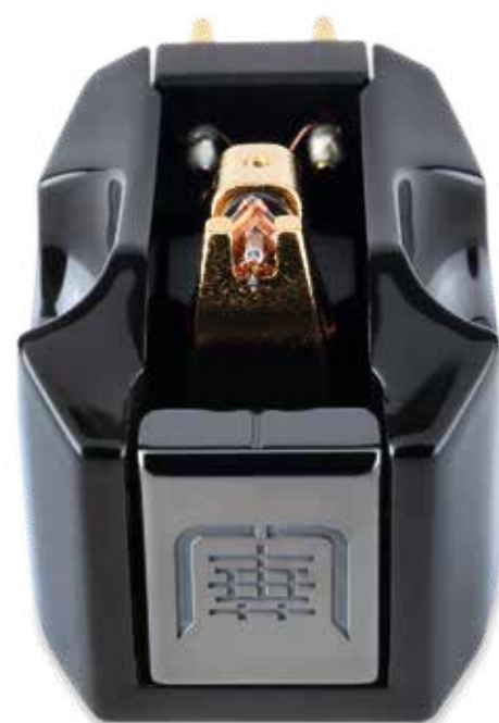
ABOVE: The Umami Black's 'OKD' generator has 4N copper coils wound onto a 2mm 2 permalloy plate/armature, seen here between the front and rear rare-earth magnet yokes
